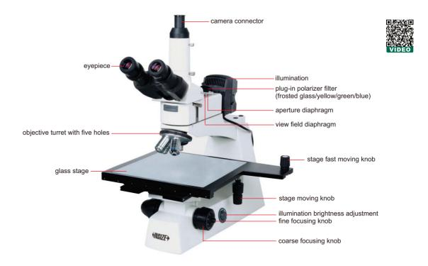
■ For observation and inspection of large IC and chip in IT industry
