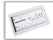
plastic calibration rule (included, graduation 1mm)
